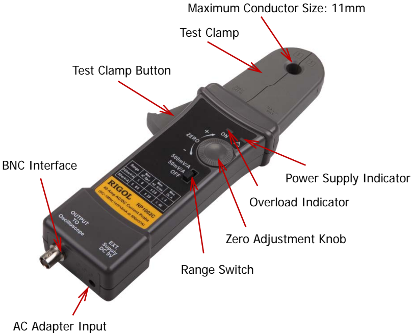
Figure 1 RP1002C Current Probe
